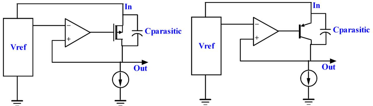
**Figure 11: Linear LDO Architecture**
