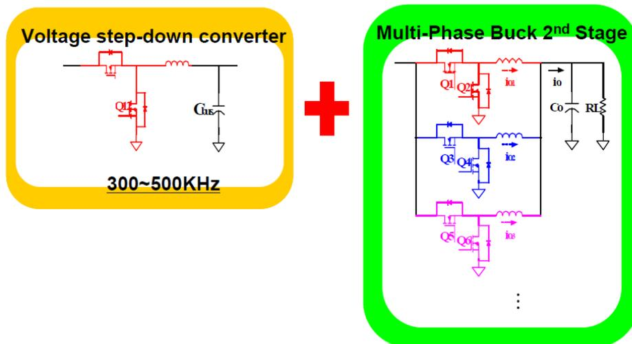
**Figure 23: Typical Buck Switching Regulators**
