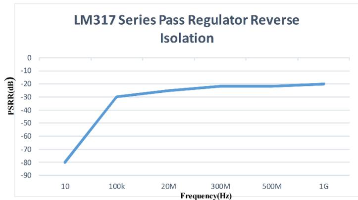
LM317 Series Pass Regulator Measured Reverse Isolation
