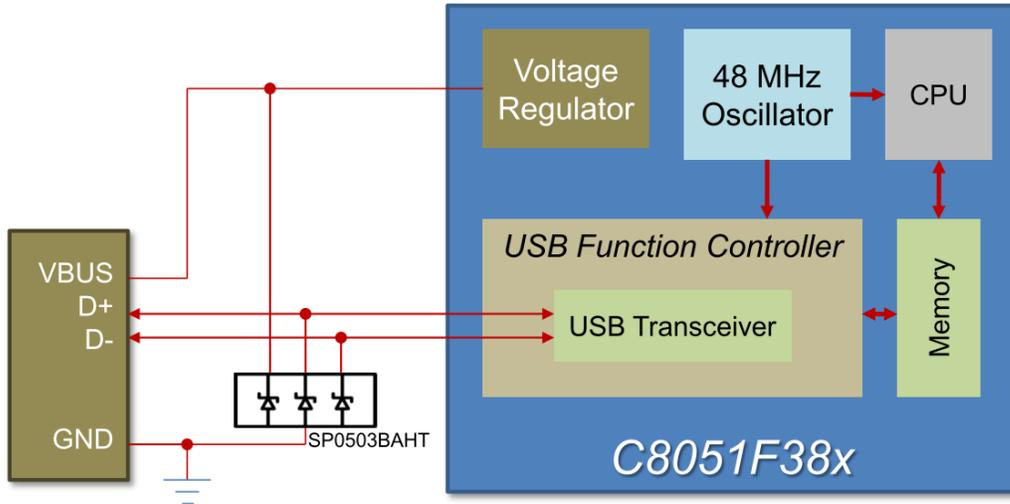
**Figure 32: Silicon Labs USB Host Controller**
