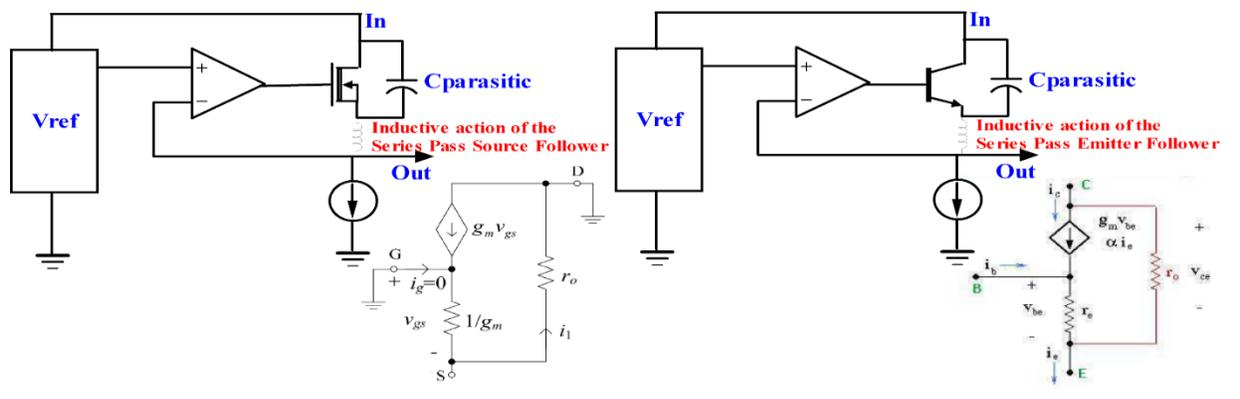
**Figure 2: Linear Series Pass Regulator Models**
