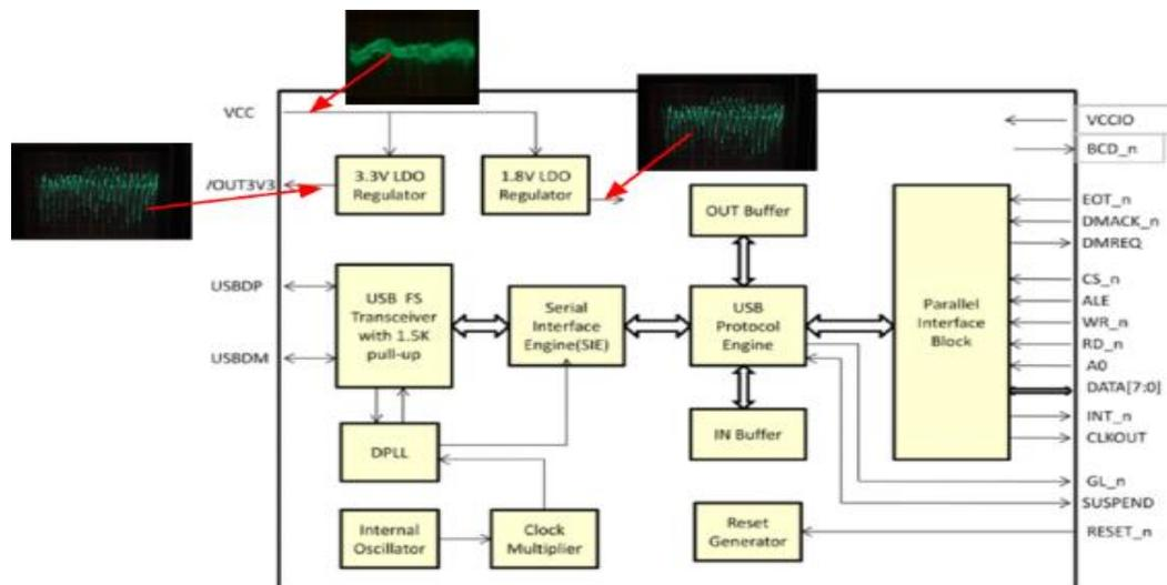
**Figure 35: FTDI USB Host Controller Reverse Coupling**
