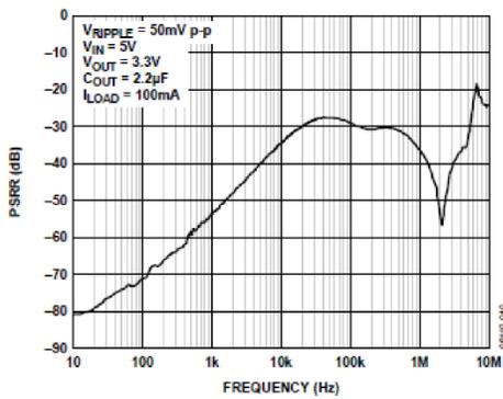
Figure 25. Power Supply Rejection Ratio vs. Frequency
