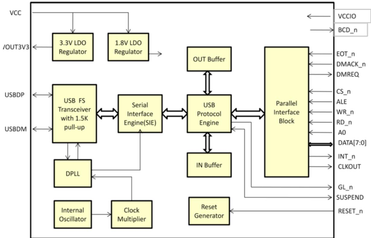
**Figure 33: FTDI USB Host Controller**
