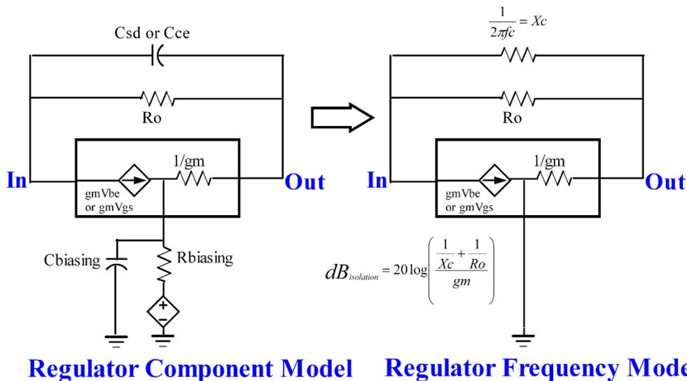
**Figure 3: Linear Series Pass Regulator Macro Model**
