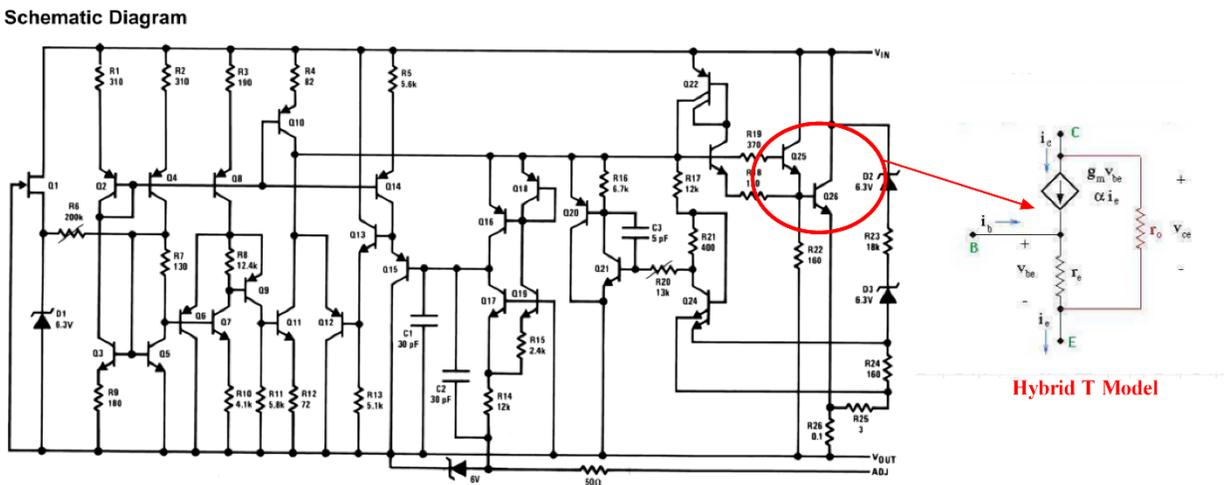
**Figure 6: LM317 Series Pass Regulator**
