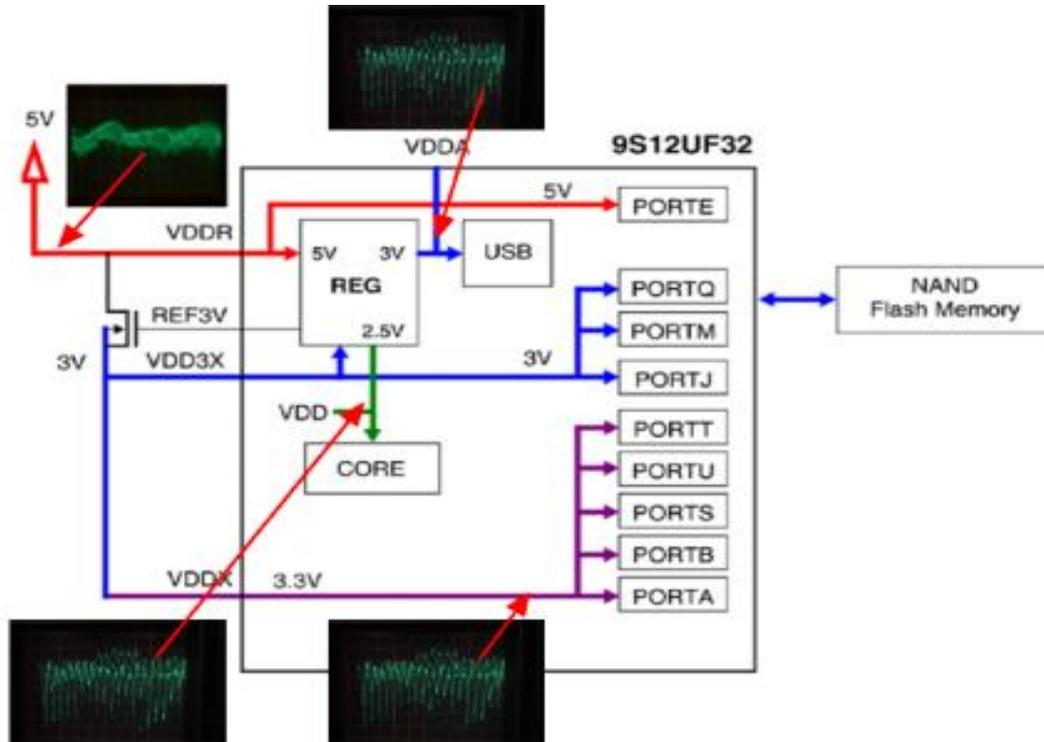
**Figure 36: Freescale Flashdrive Controller Reverse Coupling**
