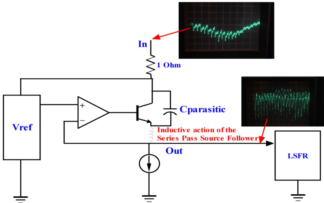
Figure 8: LM317 Series Pass Regulator Reverse Isolation Test
