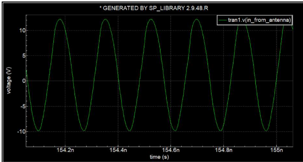
Figure 10: +33dBm Power Input at RF Rectifier Input
