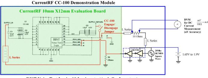
BIST Noise Test Logic=10 Logic gates(And, Or, Inverters) Typical Metrics: Supply Current- CC-100 Disengaged-----> 4.249mA Supply Current- CC-100 Engaged----> 3.774mA Delta----> .475mA Percent Reduction----> 5% to 24% Clock Rate----> 20 Mhz Supply Voltage----> 1.65 V to 1.9V
