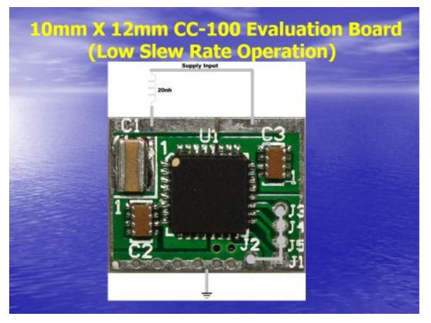
Figure 8: Low Slew Rate Operation Circuit
