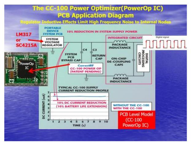
Figure 6: System Power Performance with the CC-100
