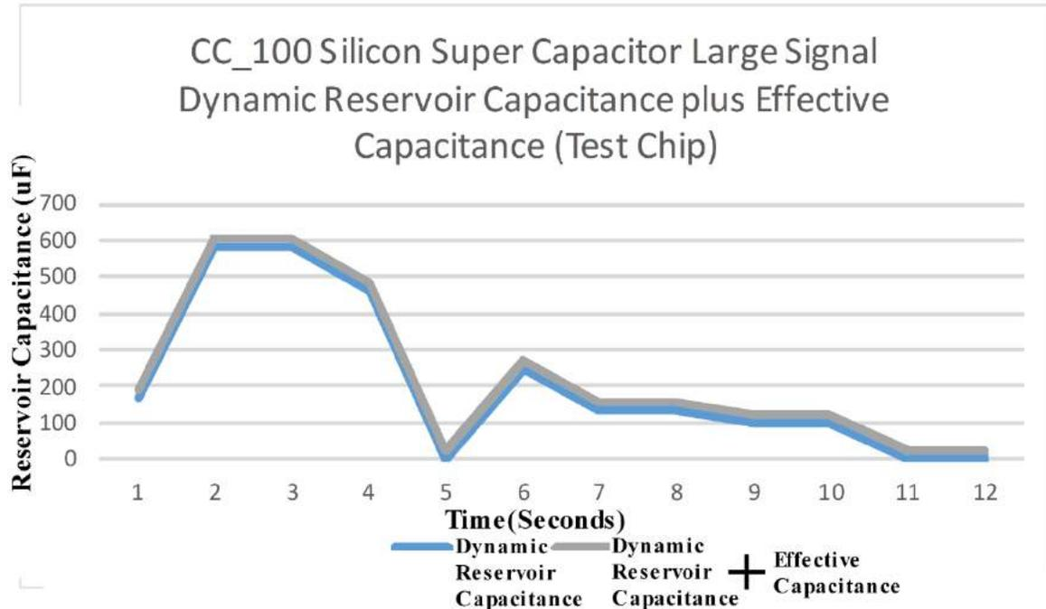
**Figure 16: CC-100IP-MB Test Chip IP Dynamic Reservoir plus Effective Capacitance Test Chip Performance (1uF Static Output Capacitance)**
