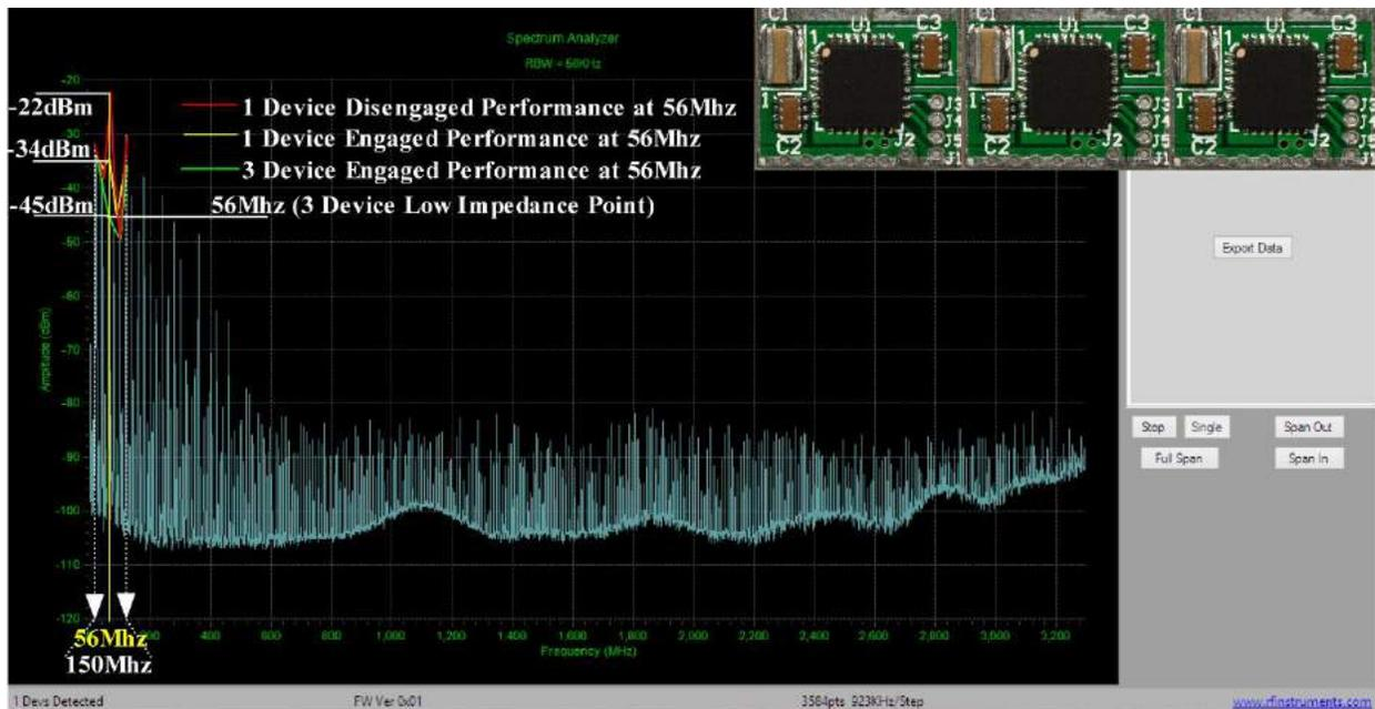
**Figure 12: CC-100IP-MB Large Signal Reservoir Capacitance Dynamics**
