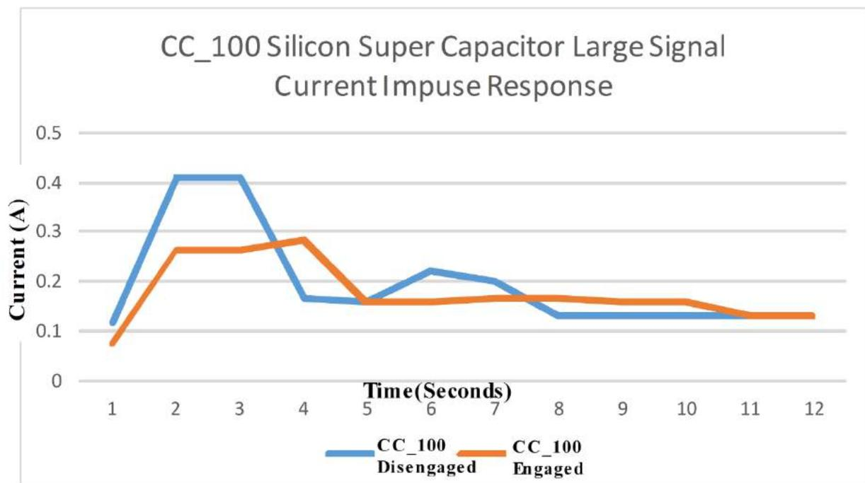
**Figure 14: CC-100IP-MB IP Disengaged/Engaged High Current Impulse Response**
