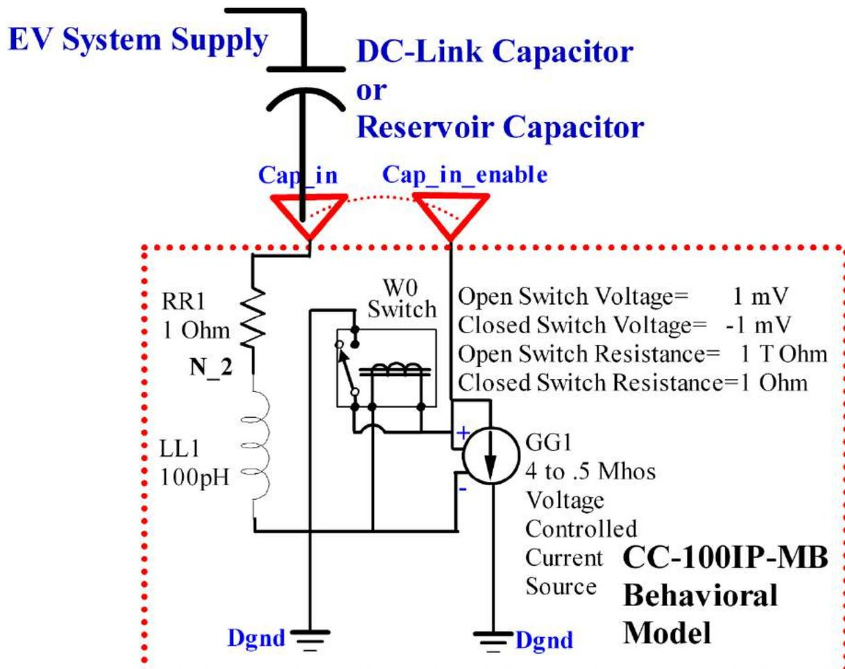
**Figure 18: CC-100IP-MB Behavioral Model Schematic and Top Level Circuit Test Bench**
