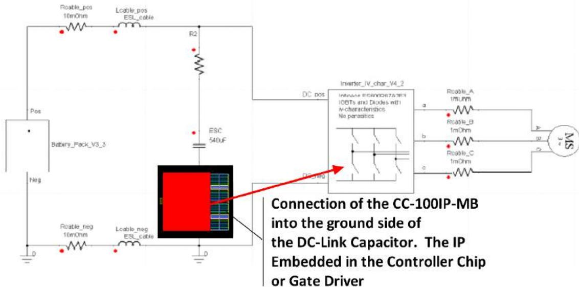
**Figure 4: Schematic for the CC-100IP-MB Controller/Traction Inverter Application**
