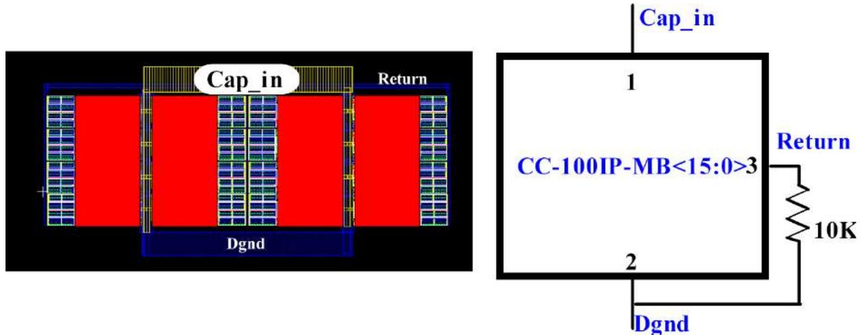
**Figure 3: CC-100IP-MB Arrayed Cell Example and Block Diagram**
