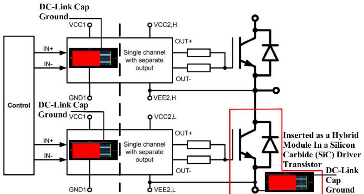
**Figure 5: Traction Inverter Gate Driver and Driver CC-100IP-MB IP insertion**
