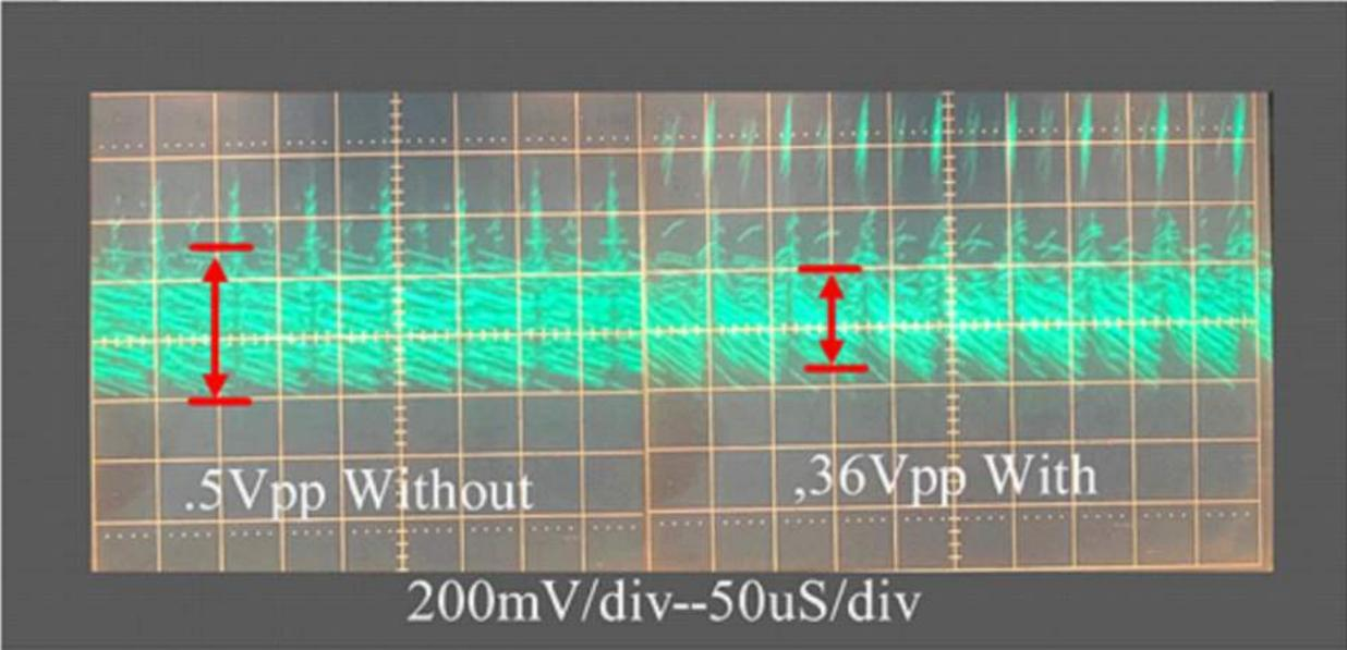
Figure 6: CC-100IP-MB E-Bike Disengaged/Engaged Time Domain Performance
