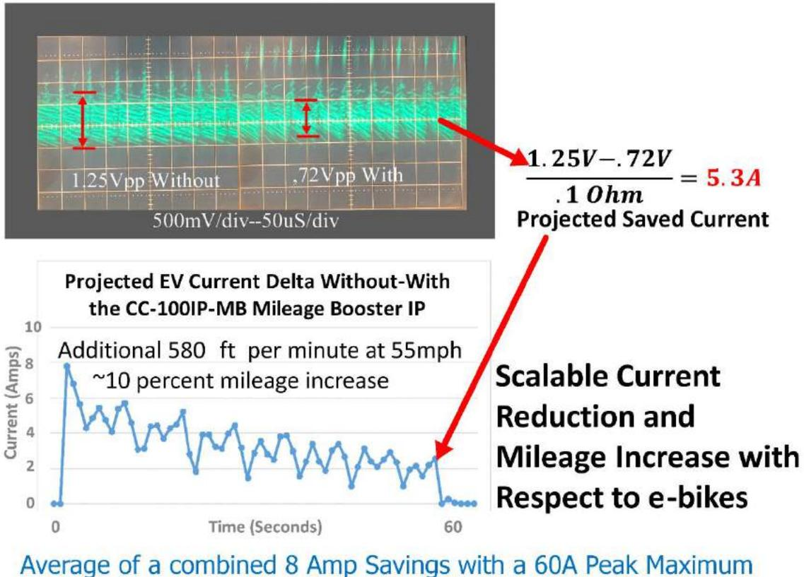
**Figure 9: EV Projected Current Savings and Mileage Increase Analysis**
