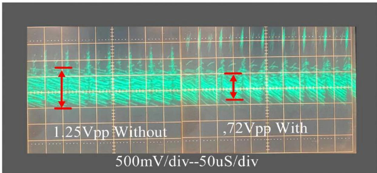
**Figure 8: CC-100IP-MB EV Traction Inverter Disengaged/Engaged Time Domain Performance**
