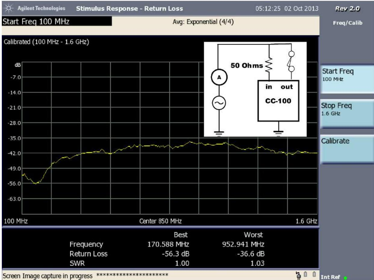
Figure 11: CC-100 IP-MB Small Signal S11 Plot (CC-100IP-MB Engaged)
