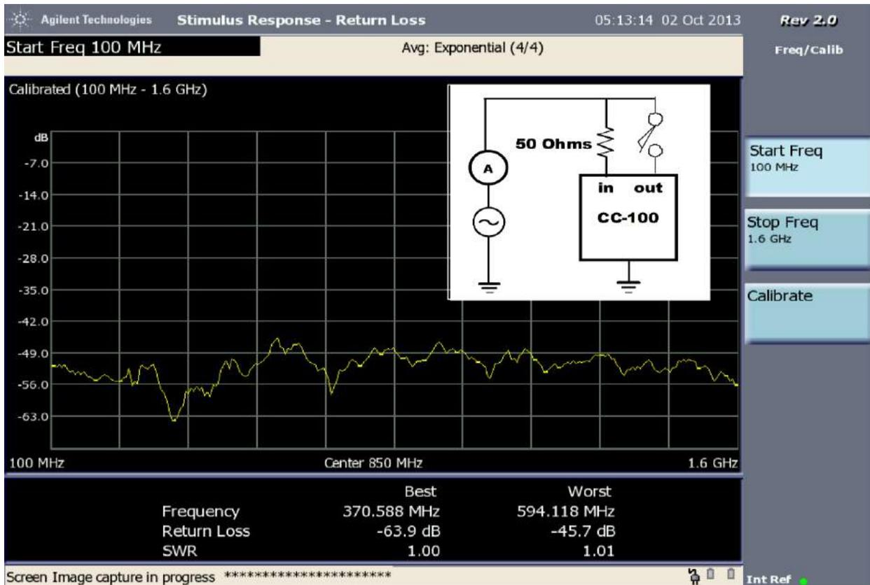
Figure 10: CC-100IP-MB Small Signal S11 Input Plot (CC-100IP-MB Disengaged)
