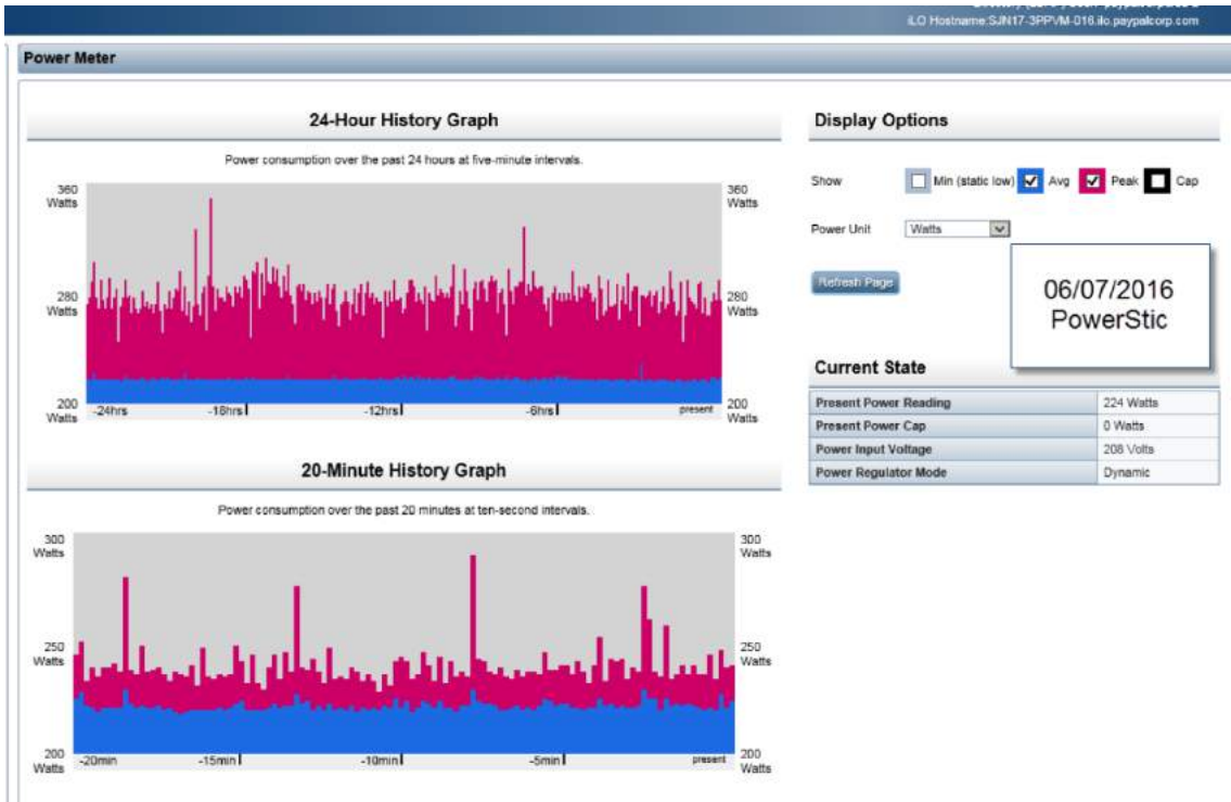
Figure 34: 24 Hour Example PowerStic-CC_100 PO/SSC IC Inserted Plot
